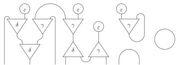
Wires can have one or both of their extremities not connected to any cell, in which case the net has a *free port*, principal or auxiliary (or neither) depending on the nature of the port of the cell connected to the other extremity of the wire. The net above has for example 7 free ports, of which 1 is principal and 4 are auxiliary. The free ports of a net are referred to as its *interface*.
