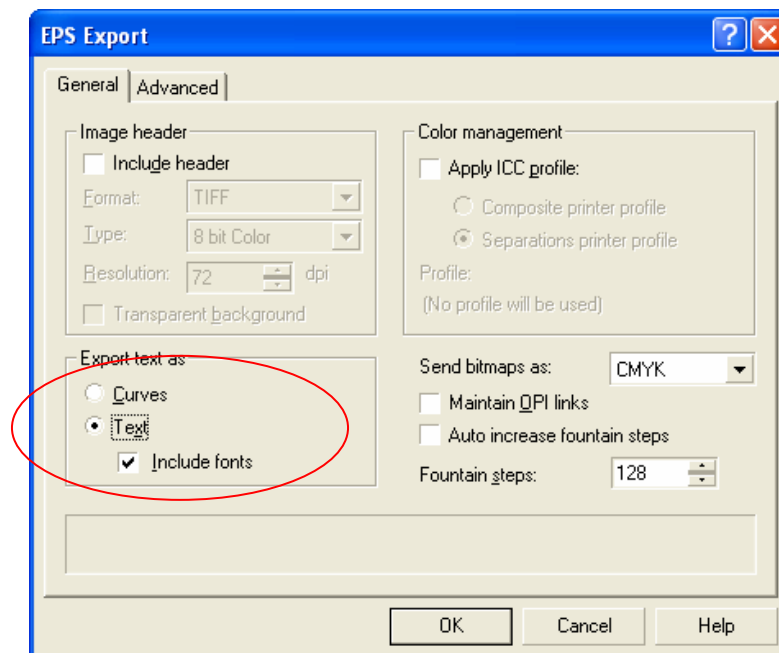
Figure 4. CorelDRAW 10's EPS Export dialog box allows you to convert text to curves or embed the font data.
